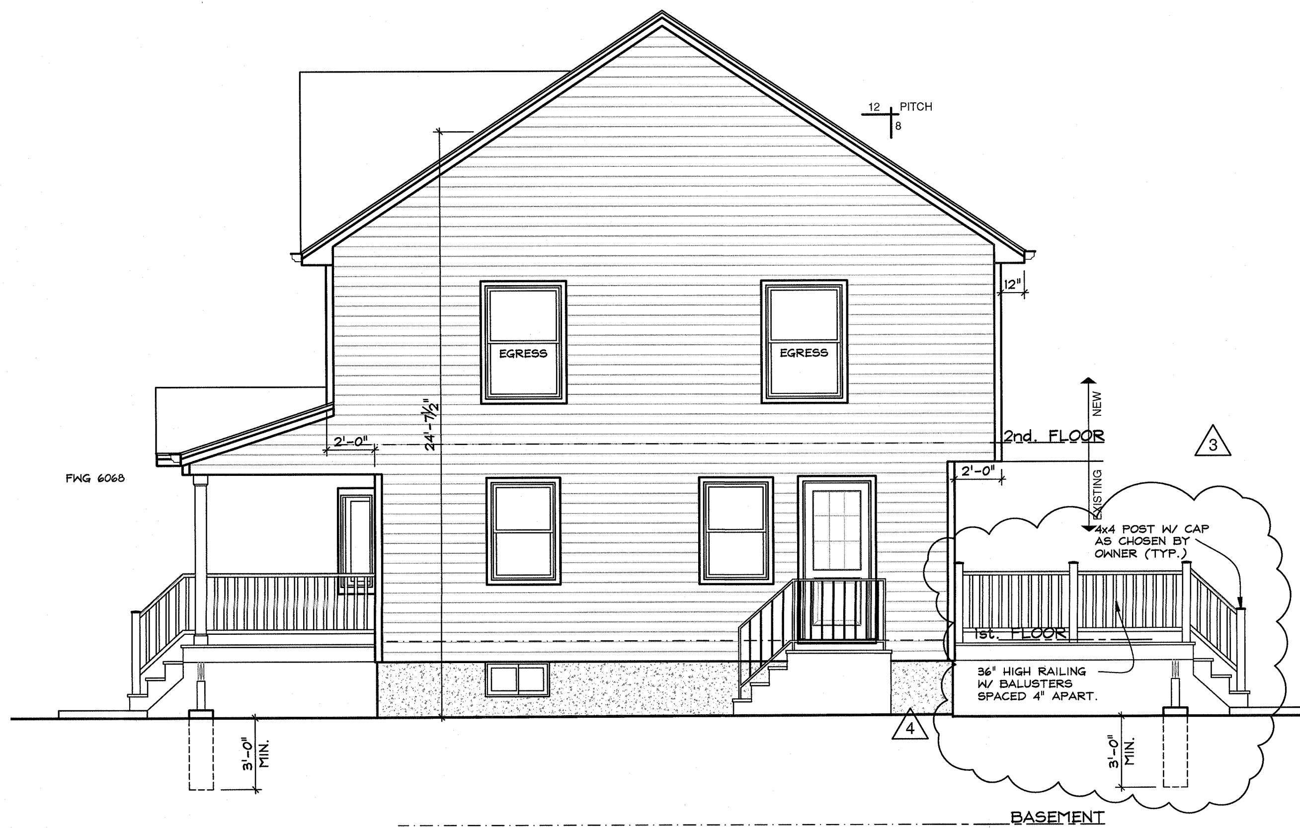
4 SIDE ELEVATION A2 1/4" = 1 FOOT
