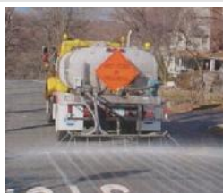
Anti-icing tanker pre-treats Orangetown roads. Photo: Orangetown Highway Dept.
