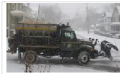
Nyack DPW plow spreads a rock salt-calcium chloride blend on snowy roads. Photo: Susan Hellauer
