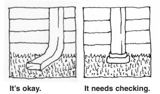
If your downspouts disappear into the ground, they may be connected to the sanitary sewer system. The water from your downspout should discharge into your yard, a storm drain or other appropriate drainage structure. Check your basement to see where the drainpipe leads. If it leads to the sewer pipe, follow these four simple steps to disconnect it.
