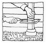
Cut the standpipe at about 9" to 10" from the ground, remove the cut piece and crimp the top piece.
