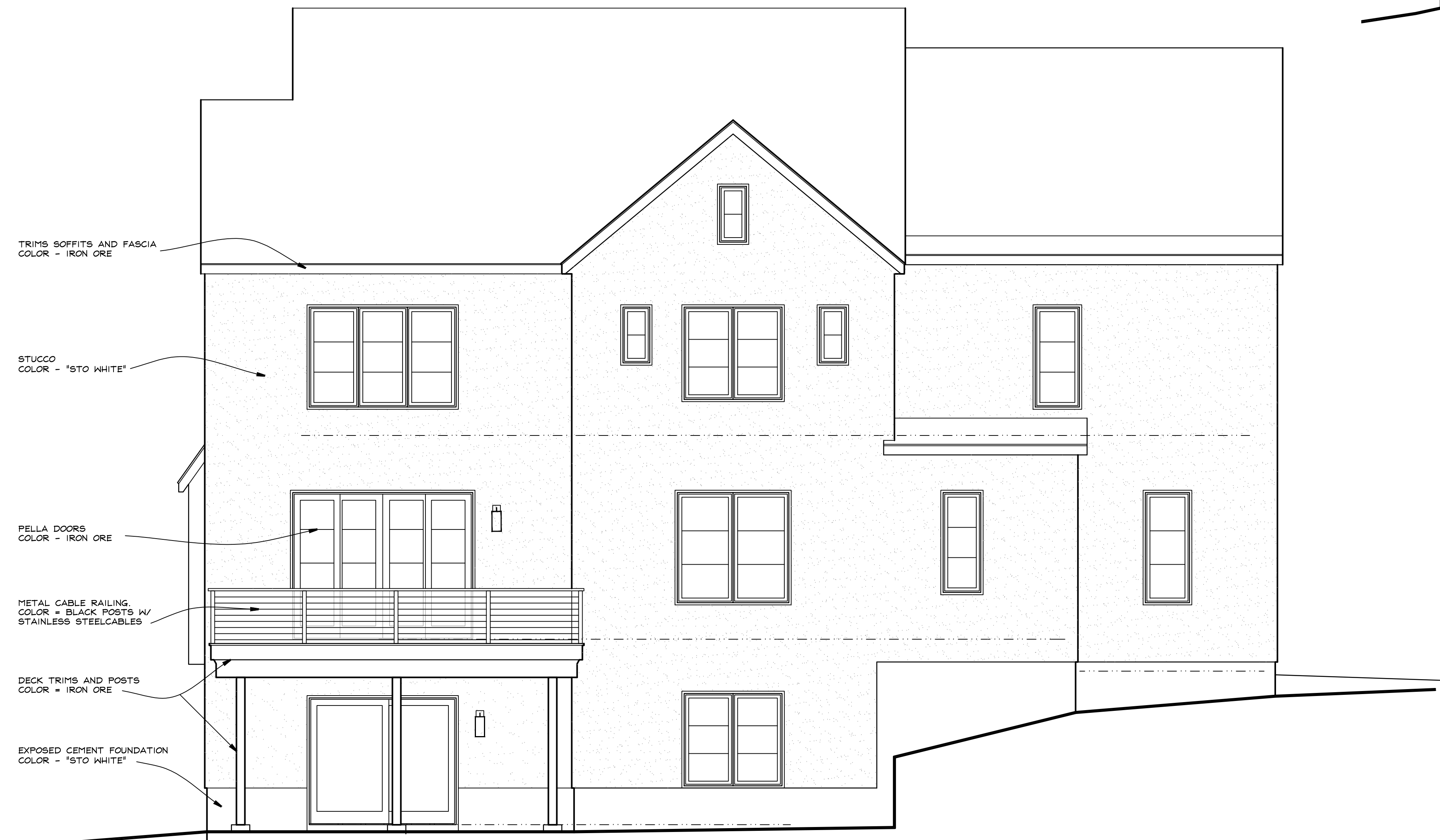
(C) REAR (EAST) ELEVATION A5 1/4" = 1 FOOT
