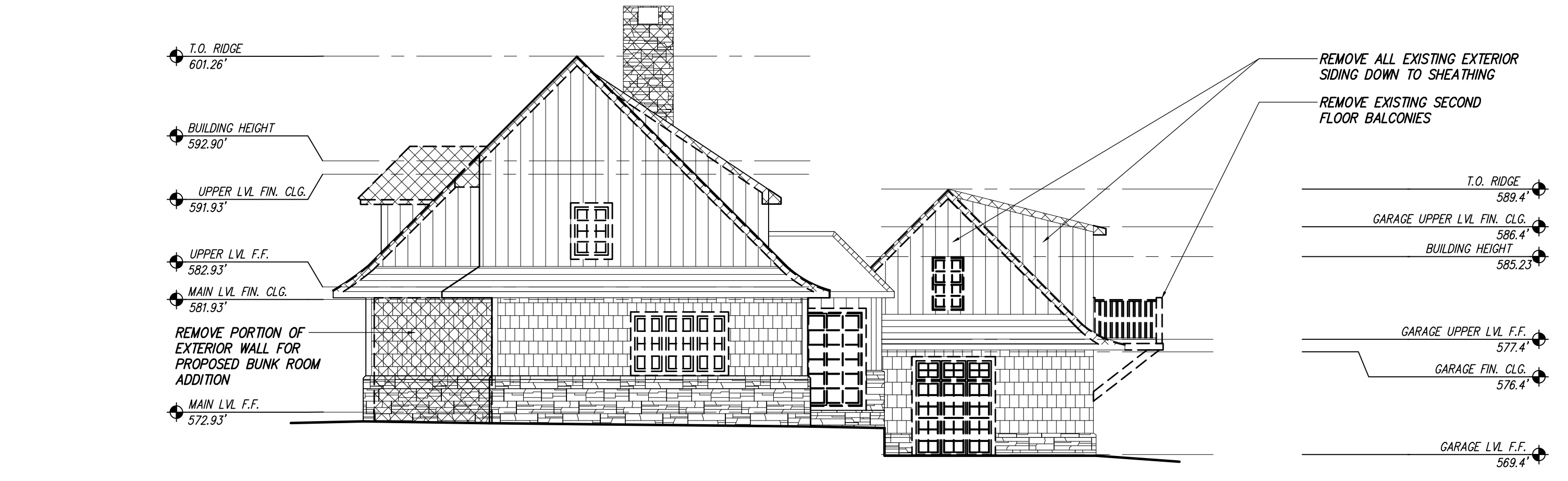
4 EXISTING SOUTH ELEVATION WITH DEMOLITION SCALE: 1/8" = 1'-0"
