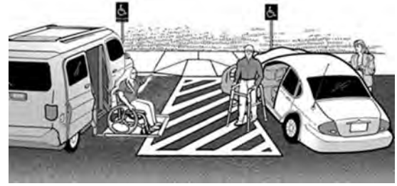
Image 9. Depiction of two accessible parking spaces sharing an access aisle
