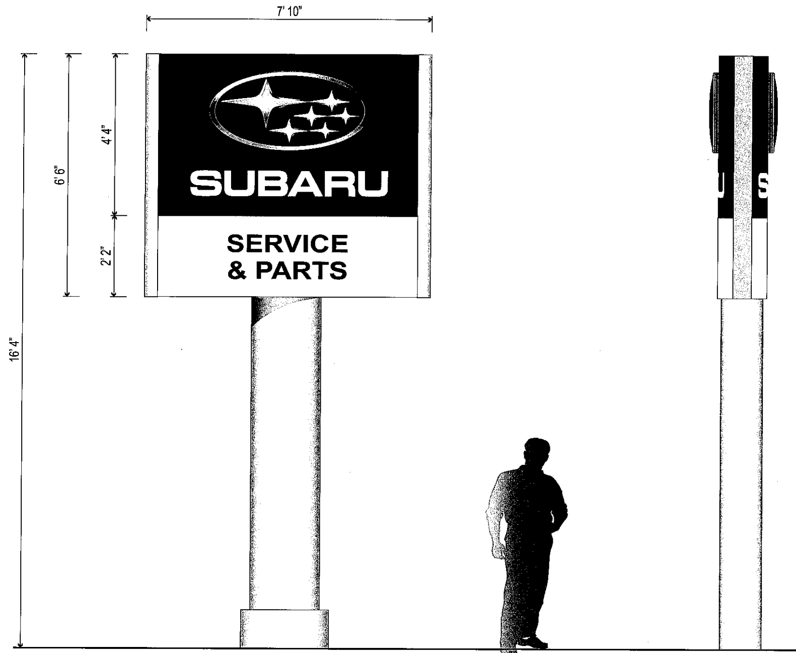
N06 - P48 2019 PYLON SIGN Scale: 3/8" = 1' 0"
