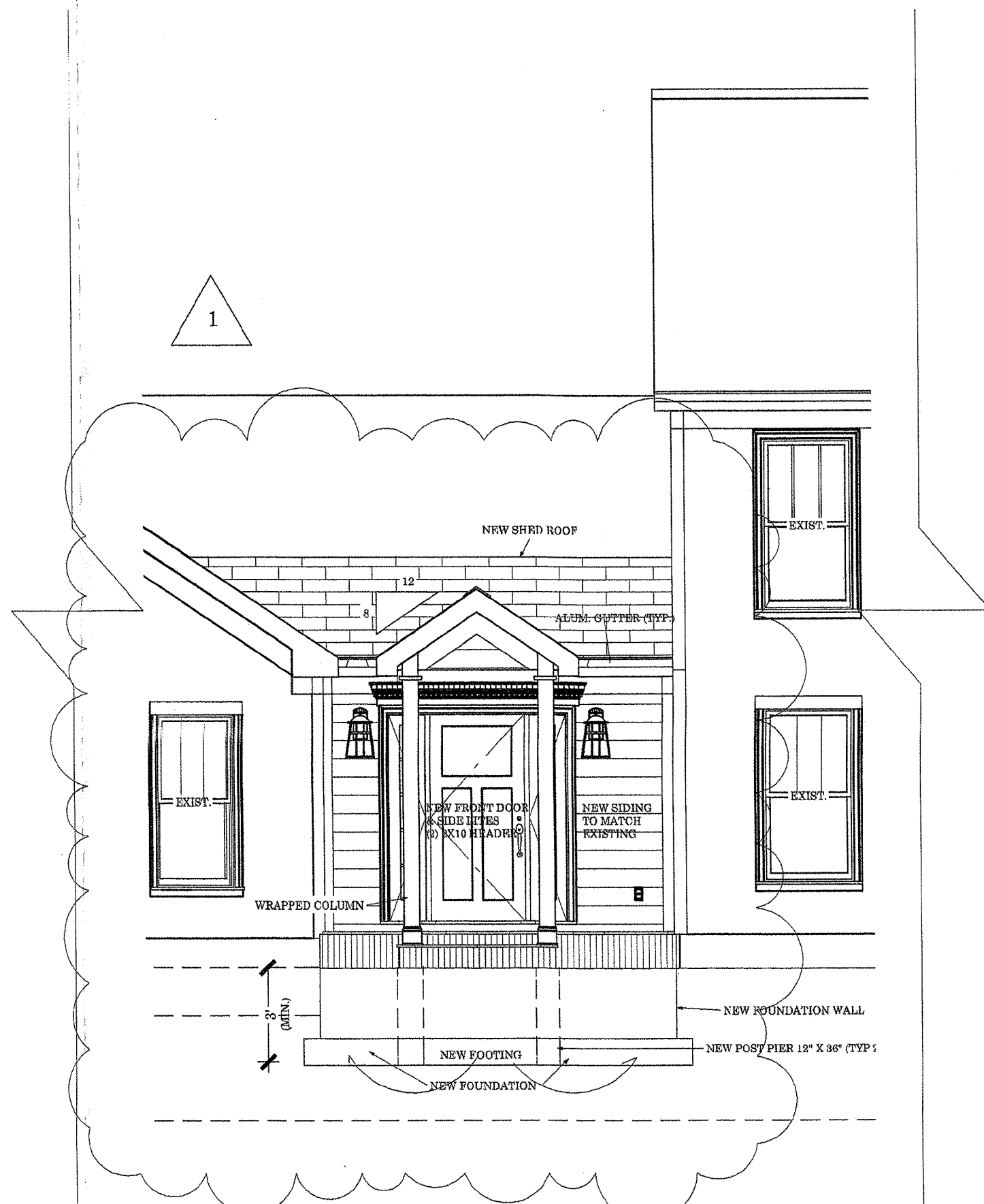
ELEVATION #1: FRONT MUDROOM ADDITION (EAST SIDE) SCALE: 1/4" = 1'-0"
