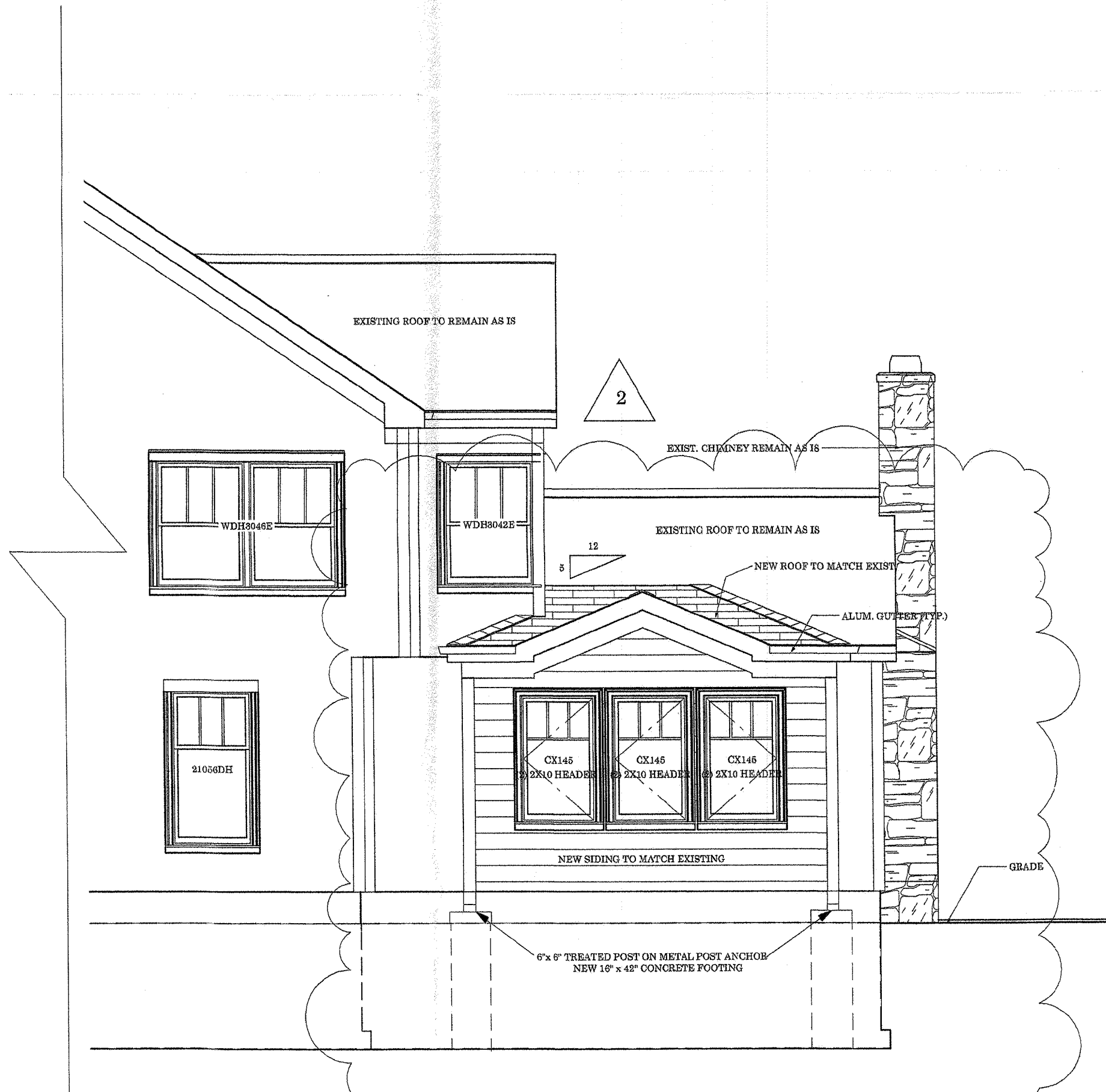
ELEVATION #1: FAMILY ROOM (NORTH SIDE) SCALE: 1/4" = 1'-0"
