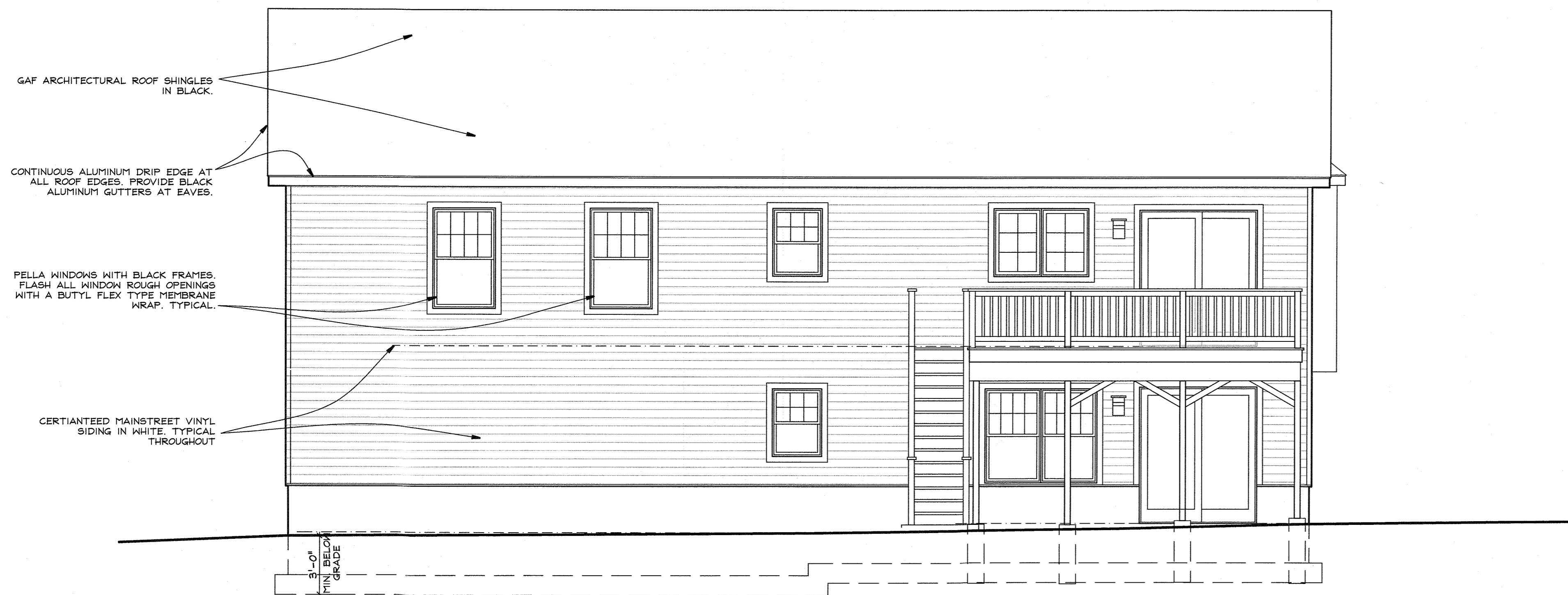
(A) REAR (NORTH) ELEVATION A5 1/4" = 1 FOOT
