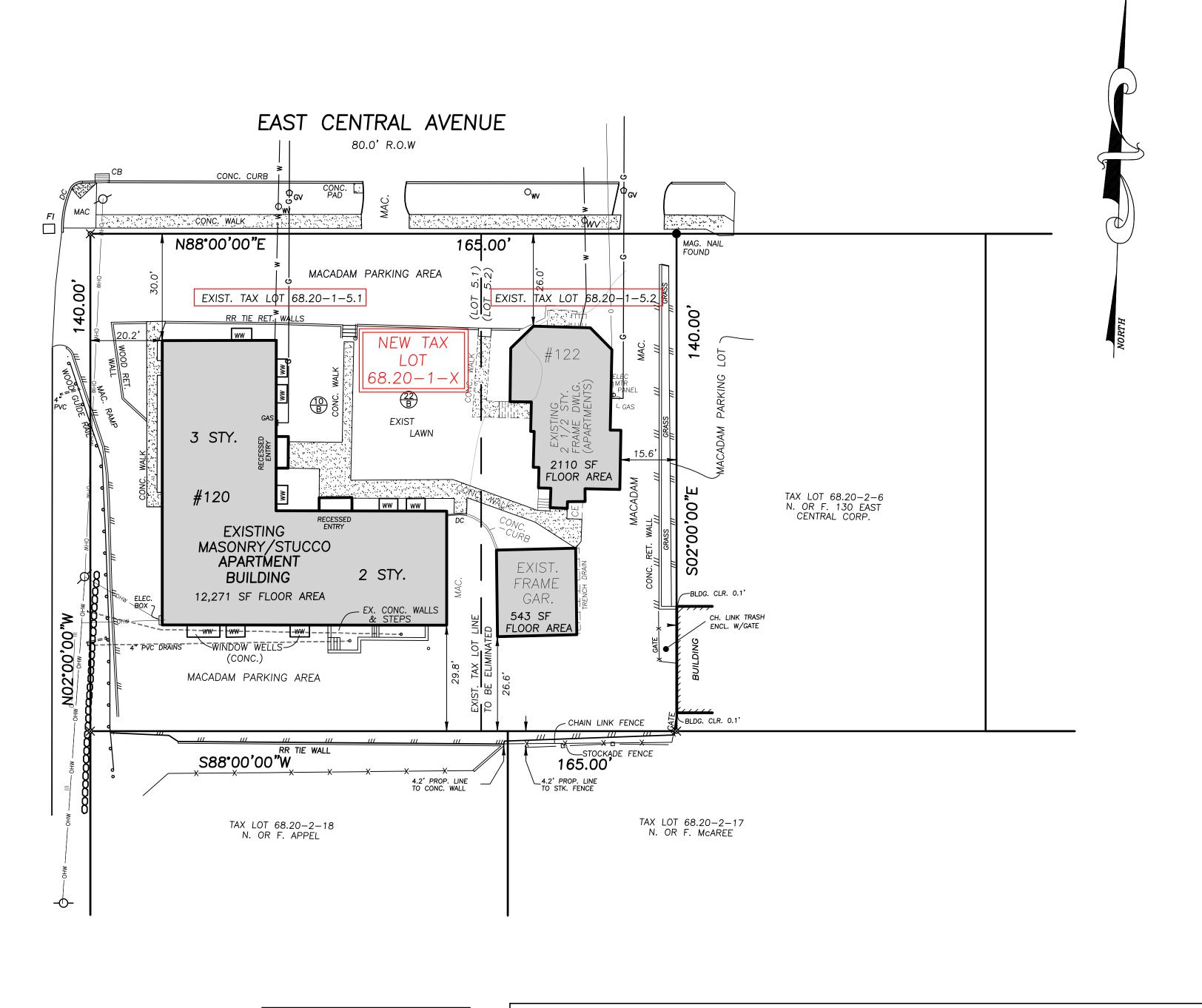
CENTRAL AVENUE FRANKLIN 19.1 SCALE 1"=20' VICINITY MAP 9. ANY EXISTING UTILITIES ( POLES, HYDRANTS, ETC.) AFFECTED BY CONSTRUCTION OF THIS SITE PLAN SHALL BE 12. ALL AREAS DISTURBED BY ON-SITE GRADING WILL BE LIMED AND FERTILIZED PRIOR TO SEEDING. 15. NO BUILDING PERMIT SHALL BE ISSUED UNTIL SITE PLANS HAVE BEEN APPROVED BY ACABOR. 16. WATER SUPPLY: UNITED WATER OF NEW YORK
