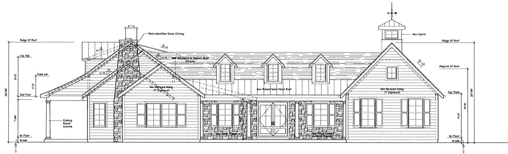
1 EXTERIOR ELEVATION - FRONT SCALE: 3/16" = 1'-0" EAST FACADE
