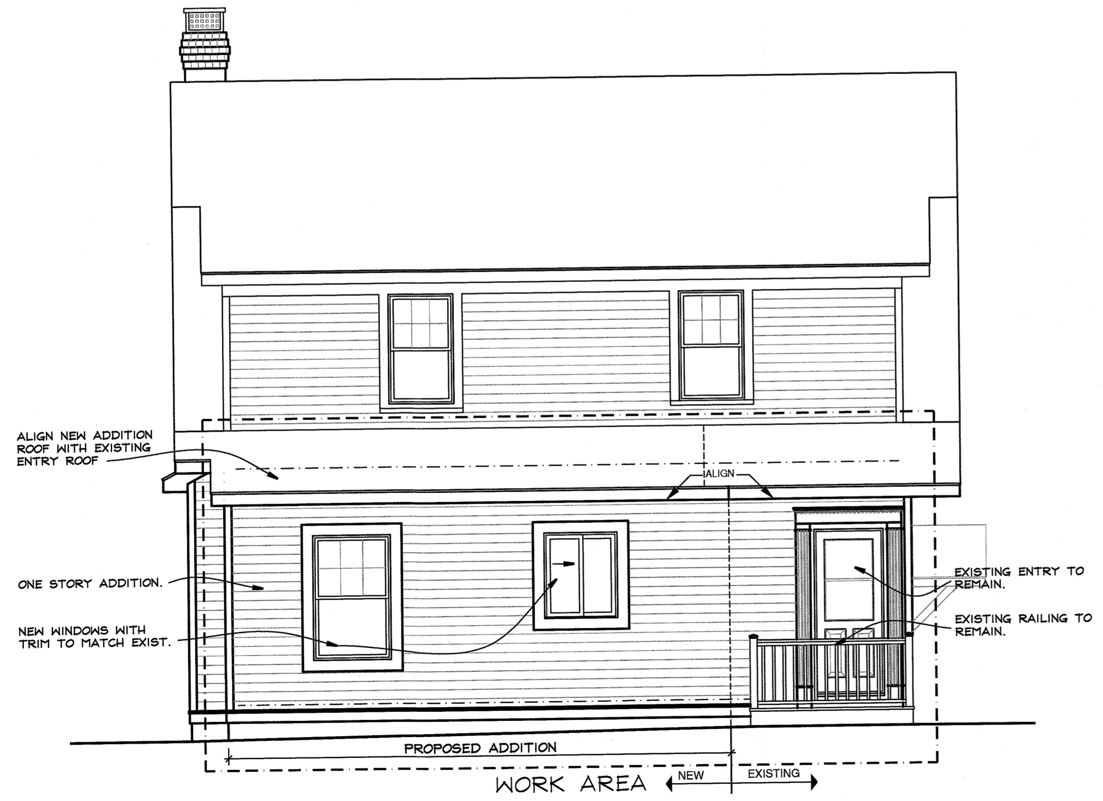
2 WEST ELEVATION 1/4" = 1 FOOT
