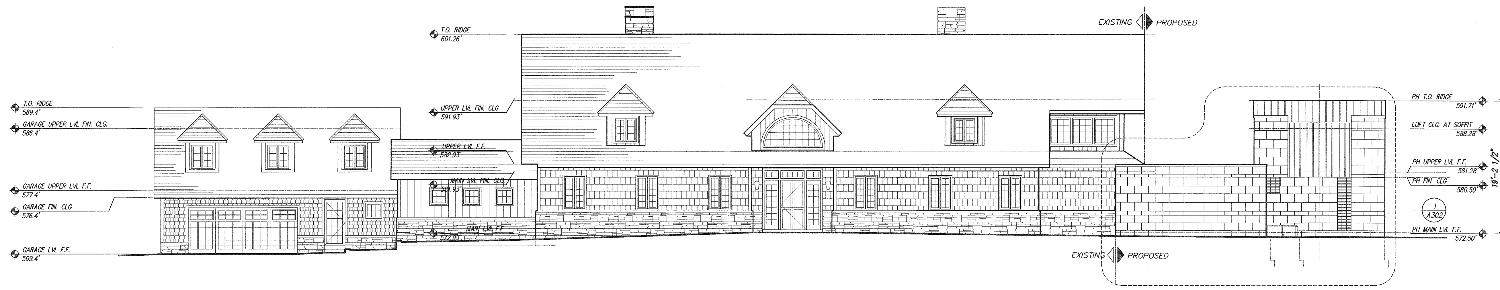
1 PROPOSED WEST ELEVATION A301 SCALE: 1/8" = 1'-0"
