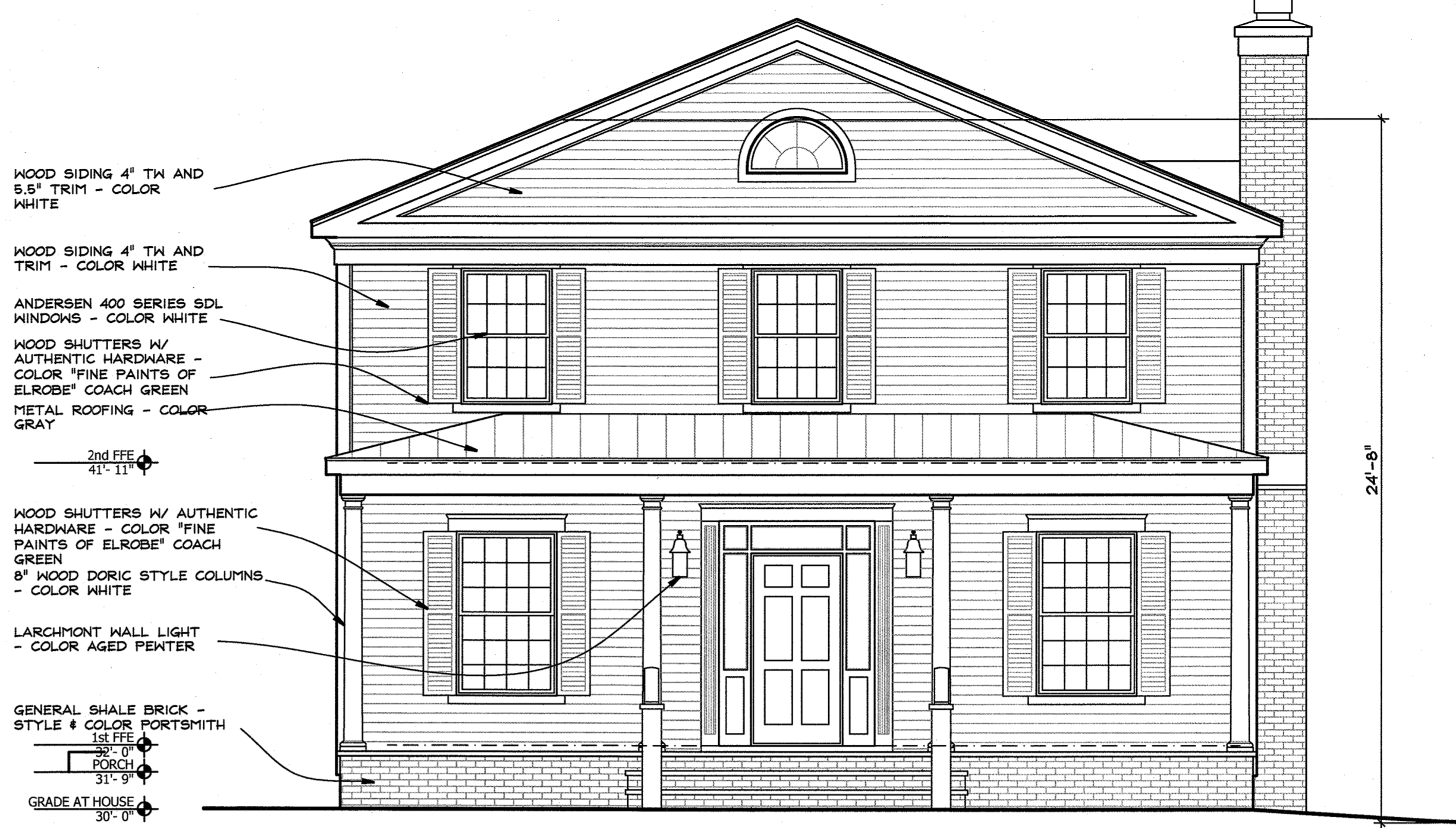
(A) FRONT (SOUTH) ELEVATION A3 1/4" = 1 FOOT
