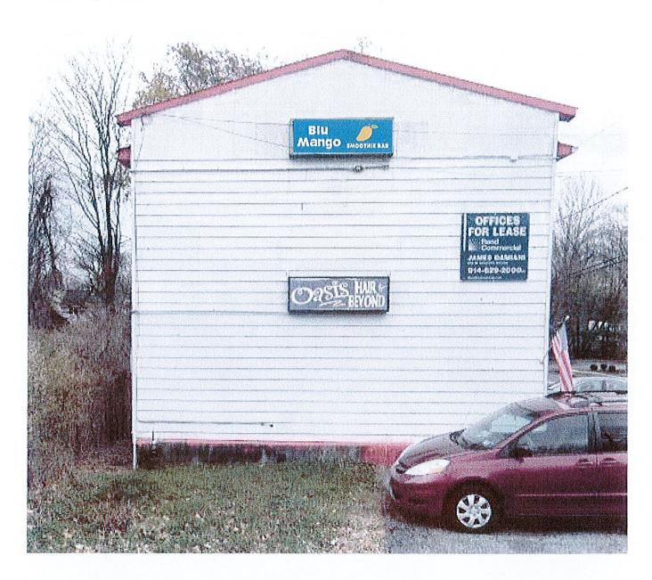
REFACE EXISTING LIGHT BOX FOR SIGN WITH  $\frac{1}{2}$ " OUTDOOR PVC,  $\frac{2}{2}$ 6' DIGITAL PRINT, LAMINATED. MOUNTED ON EXISTING LIGHT BOX WITH SCREWS.
