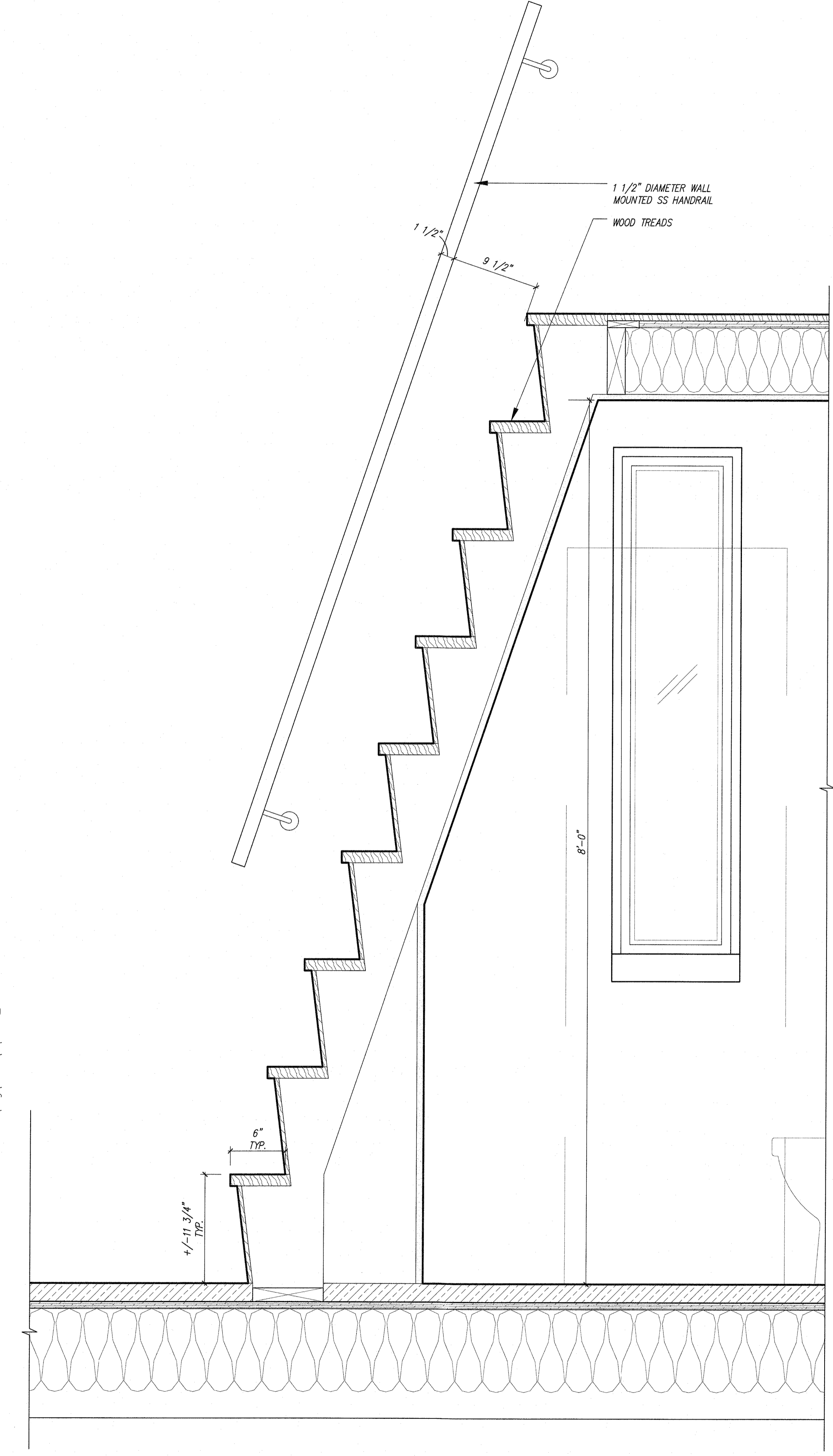
4 PROPOSED SECTION THROUGH POOL HOUSE STAIR SCALE: 1-1/2" = 1'-0"
