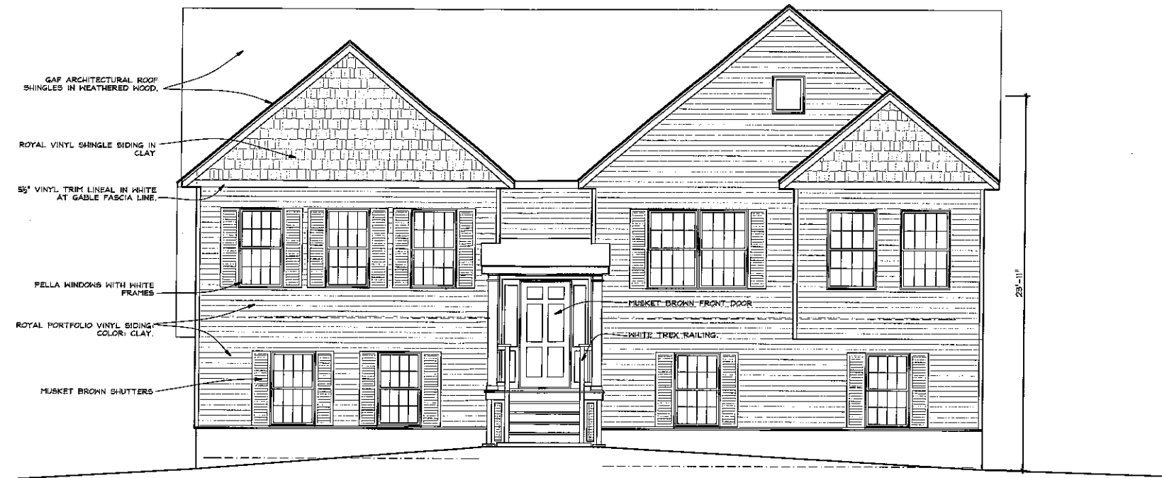
(A) FRONT (NORTH) ELEVATION A4 1/4" = 1 FOOT
