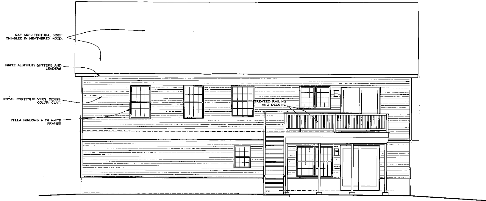
Ⓒ REAR (SOUTH) ELEVATION A4 1/4" = 1 FOOT
