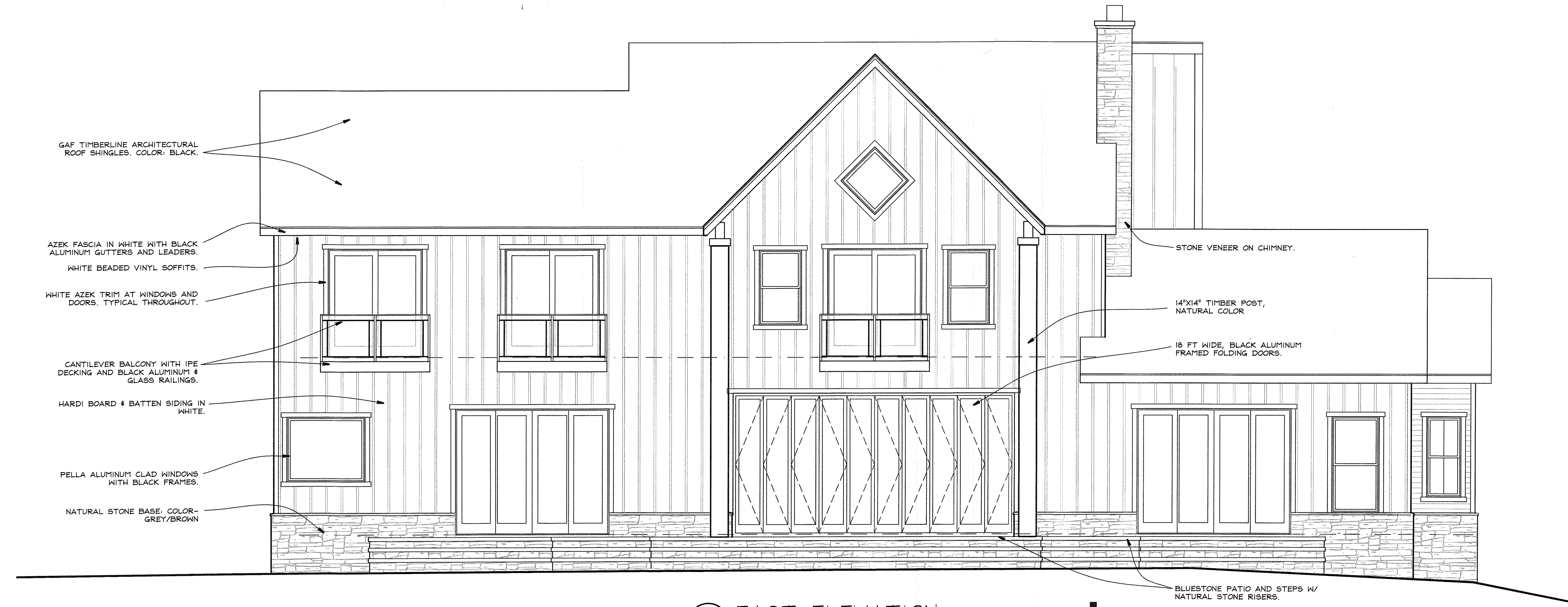
D EAST ELEVATION A5 1/4" = 1 FOOT
